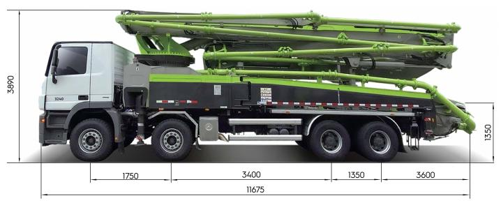
**Note:** Standard version. Dimensions and weights depend on truck, pump model and equipment. Dimensions are in mm. Example based on Mercedes-Benz Arocs 5 3240 8 x 4. For illustration only. Actual products may vary.
