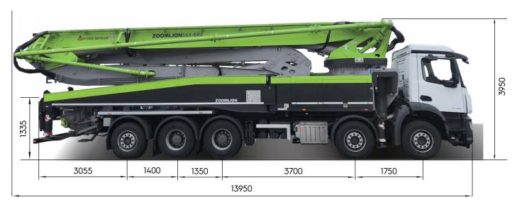
**Note:** Standard version. Dimensions and weights depend on truck, pump model and equipment. Dimensions are in mm. Example based on Mercedes-Benz Arocs 5 5246. For illustration only. Actual products may vary.
